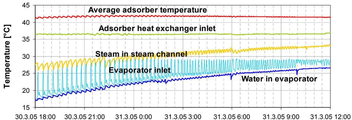
**Figure 6: Adsorption test with constant adsorber temperature**
