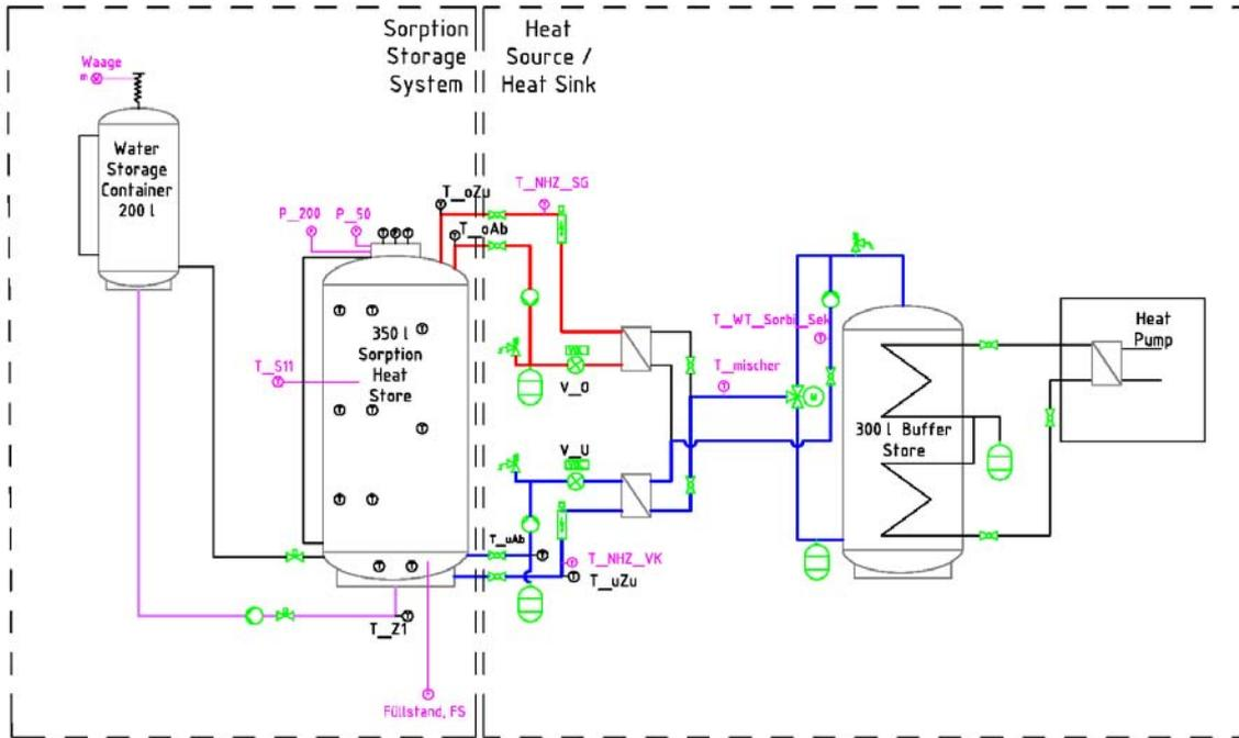
Figure 3: Setup of the test facility
