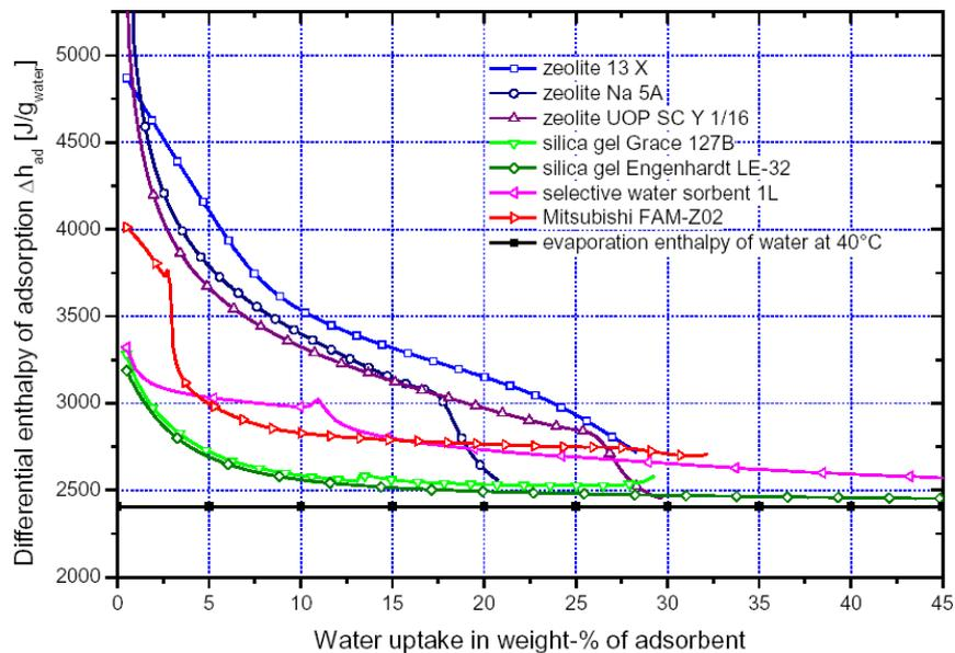
**Figure 7: Differential heat of adsorption vs. water content of adsorbent from Hadorn (ed.), 2005**
