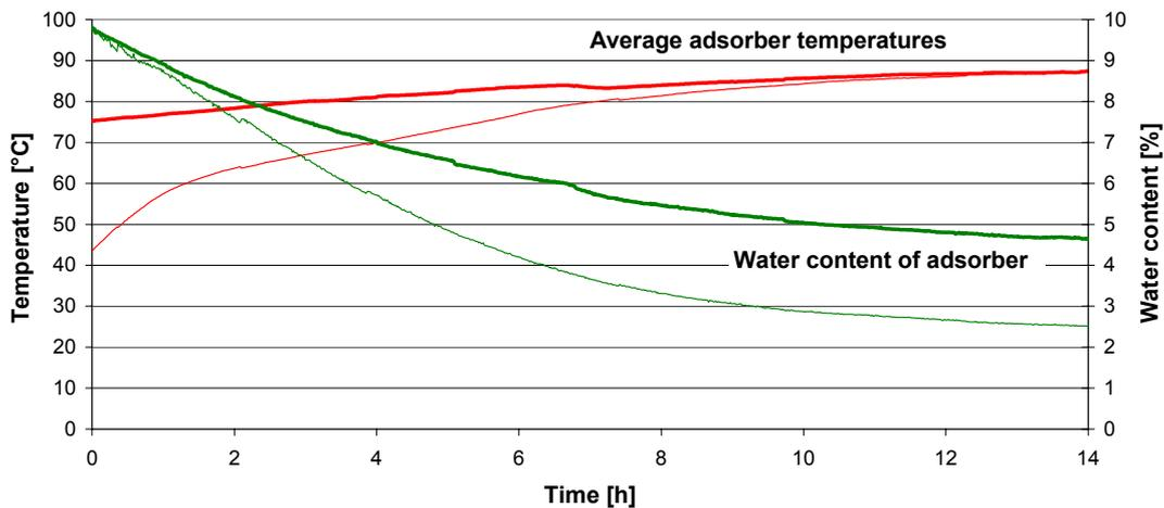
**Figure 4: Desorption with two different condensation temperatures**
