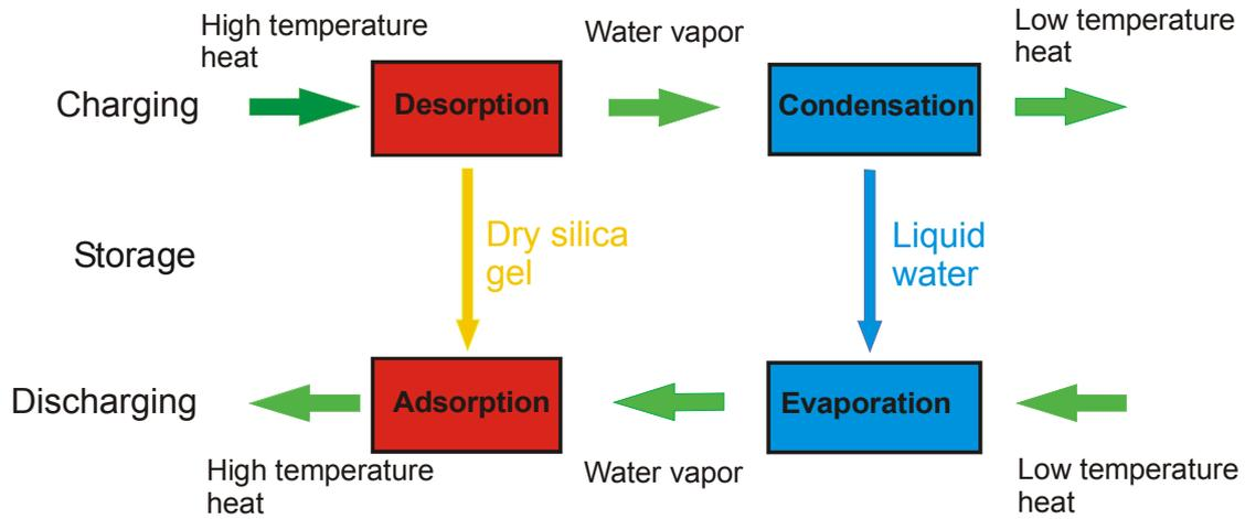
**Figure 1: Working principle of a closed-cycle adsorption heat store**
