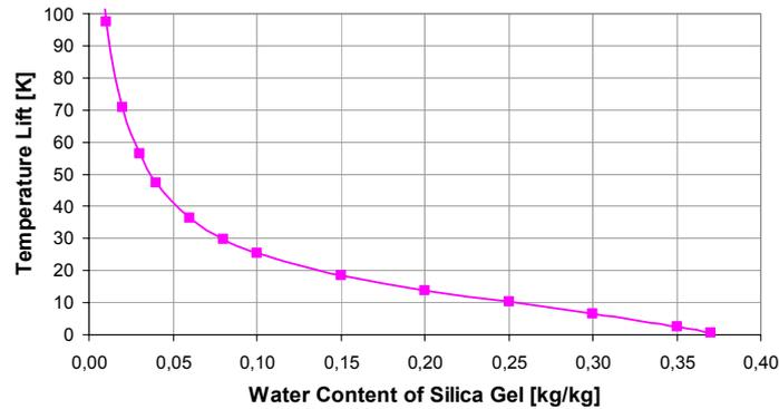
**Figure 5: Available temperature lift as a function of water content of the silica gel at an evaporator/condenser temperature of 20°C**
