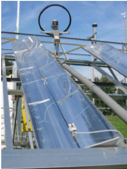
Figure 3: Parabolic trough collector under development at AEE INTEC in Austria
