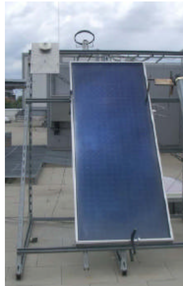
Double glazed collector with AR-glasses on outdoor testsite of Fraunhofer ISE, Germany
