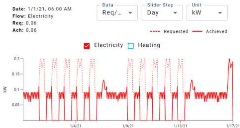
Figure 5-12. Facility IONL cannot meet loads during times of peak consumption.
