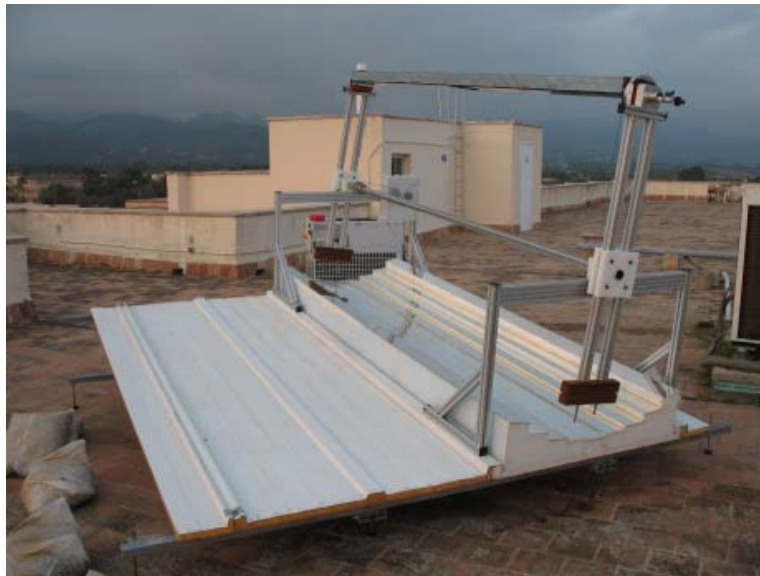
The CCStaR collector developed by the Universitat de les Illes Balears, Spain
