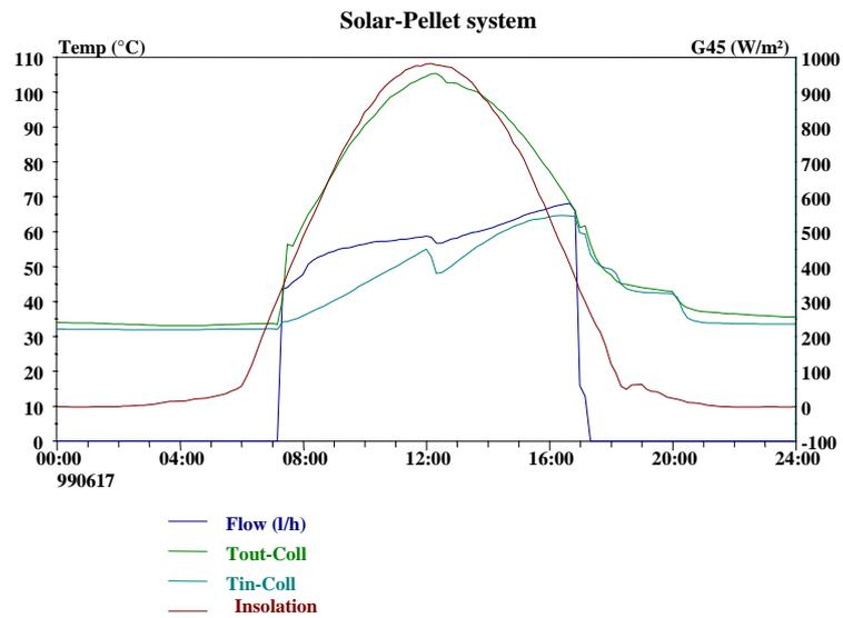
Fig. 4 The diagram shows the daily input/output from the collector
