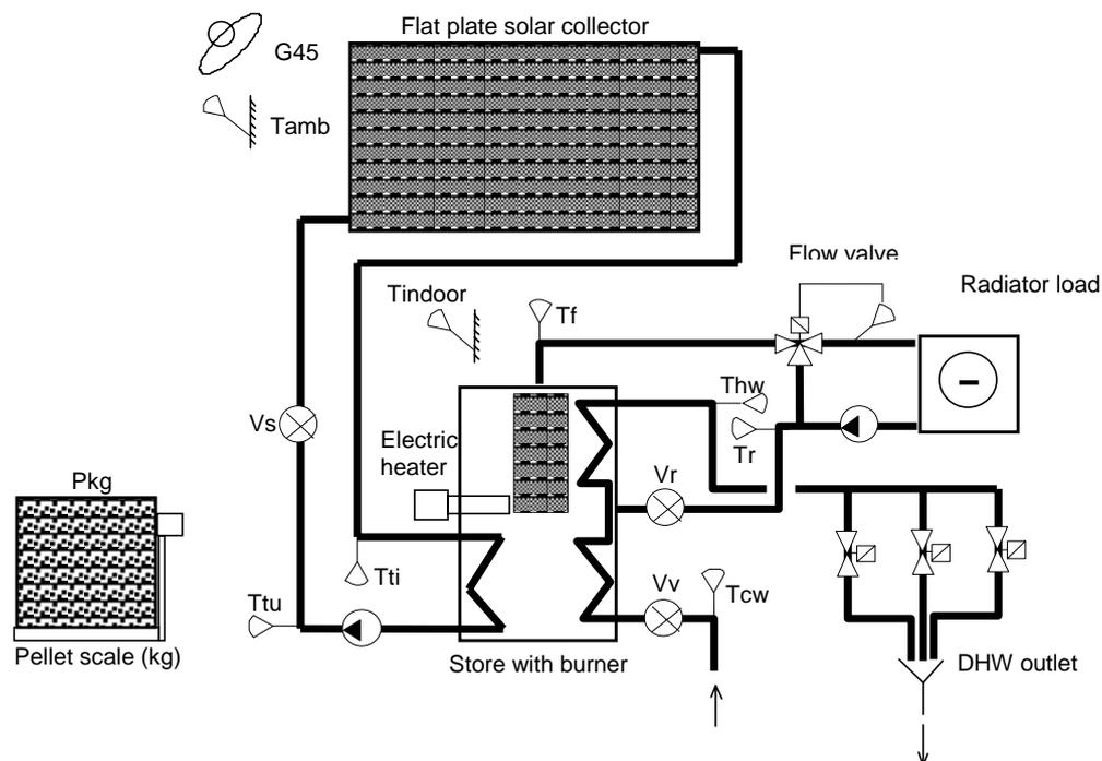
Fig. 1 Principle drawing of the system with sensors included
