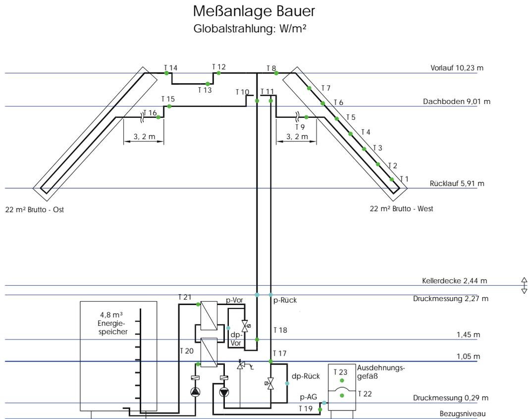
*Fig. 1: Hydraulic and measuring concept of a plant with a collector area of 44 m<sup>2</sup> and an energy storage tank volume of 4,5 m<sup>3</sup>.
