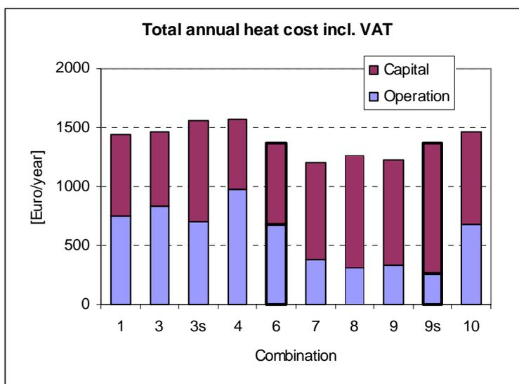
Fig. 6 Total annual cost with annuity 0.07, pellet price 0.03 Euro/kWh and electricity price 0.09 Euro/kWh for combinations shown in Table 1 complemented with two solar alternatives, 3s and 9s, replacing comb. no 2 and 5.
