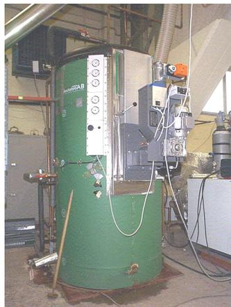
Fig. 8: The final prototype used in the test with the burner
