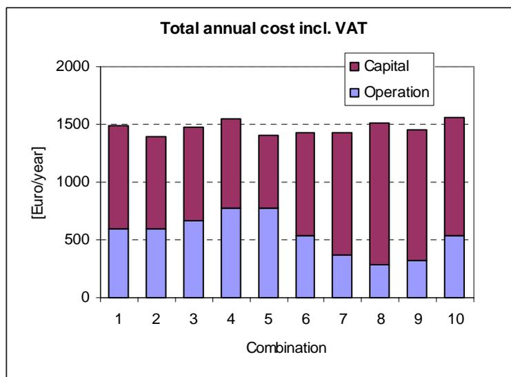
Fig. 5: Total annual costs using annuity 0.09, pellet price 0.03 Euro/kWh and electricity price 0.07 Euro/kWh for combinations shown in Table 1.
