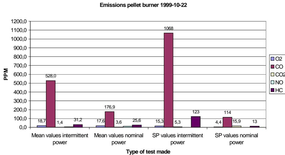
Fig. 5 The diagram shows results from pellet burner emission tests.
