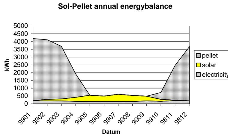
Fig 3. Diagram shows the annual energybalance of the system during the period
