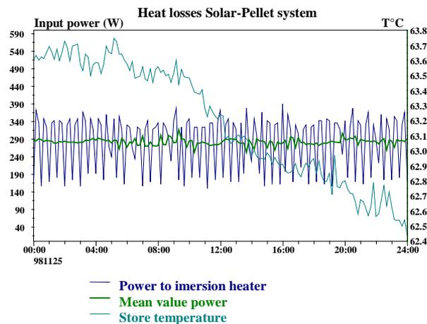
Fig. 7 Store heat losses at 45 degrees  $\Delta t$  ( $^{\circ}K$ )
