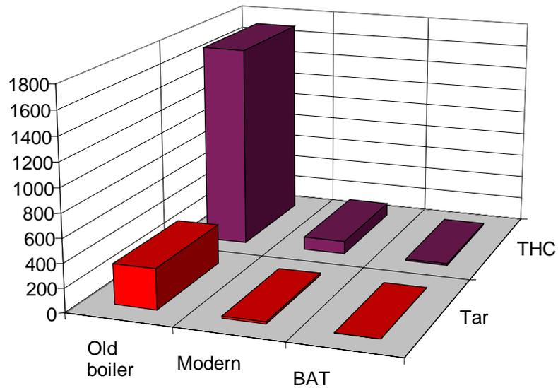
Fig. 1: Comparison of emission from different types of wood boilers
