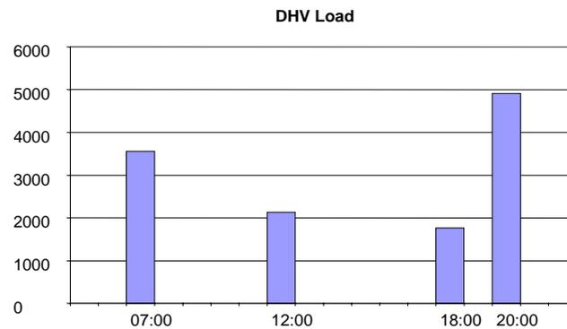
Fig.2 Daily DHW load used in the setup (i.e. 4 individual tappings per day).
