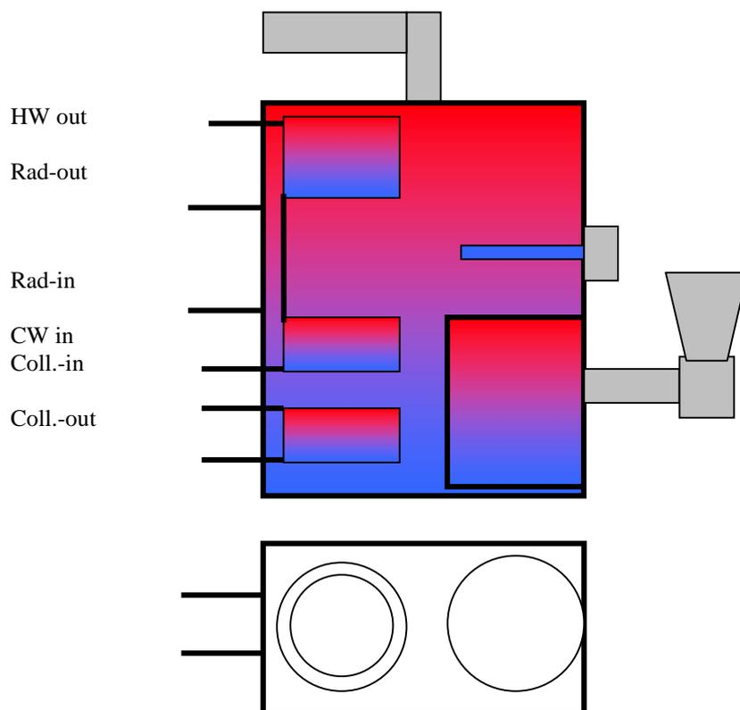
*Fig. 1 Pellet boiler with integrated heat exchangers for the solar circuit and domestic hot water preparation.*
