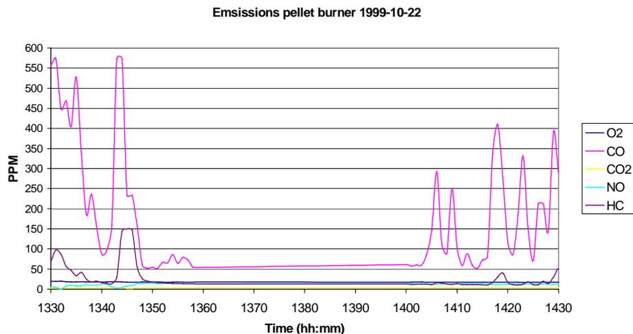
Fig. 6 The diagram shows emissions during different types of load with on/off control strategy
