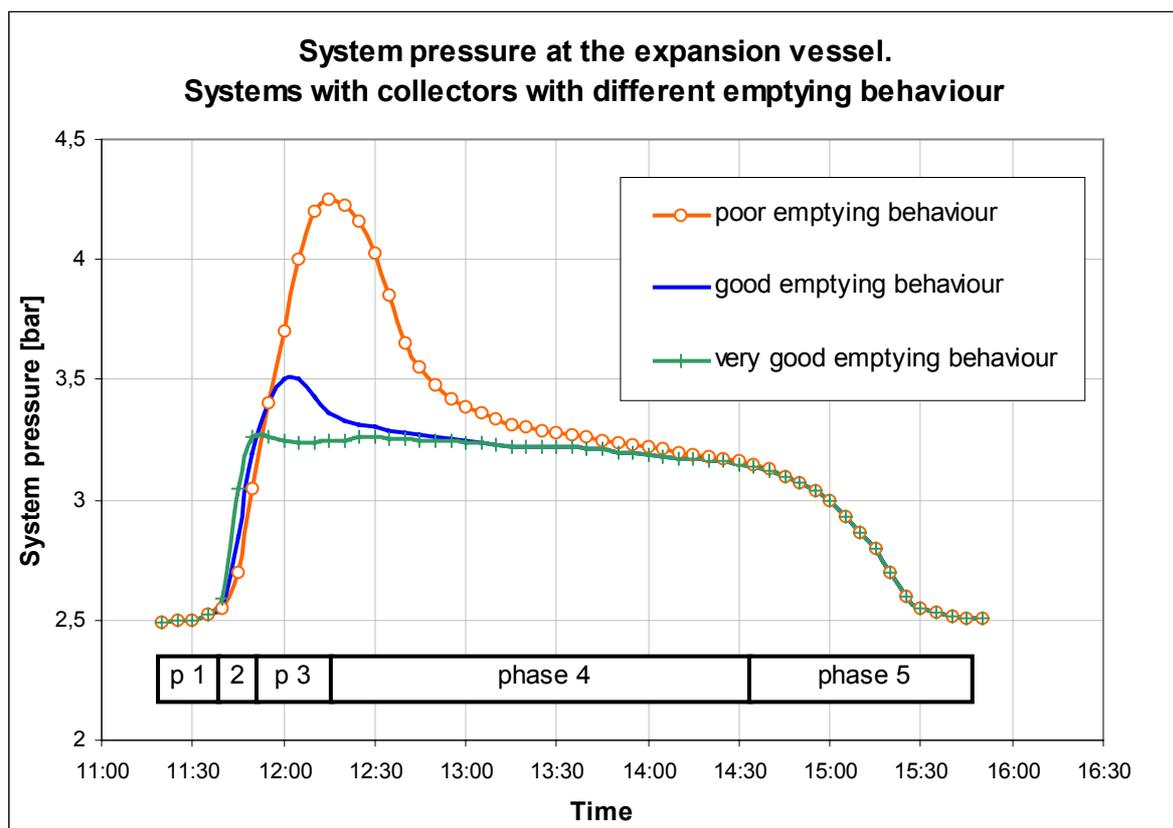
Figure 1: System pressure versus time for three different emptying behaviours.
