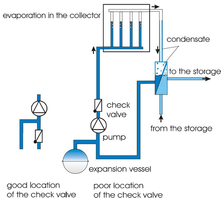
Figure 6: Good and poor arrangement of the components of the primary solar circuit..
