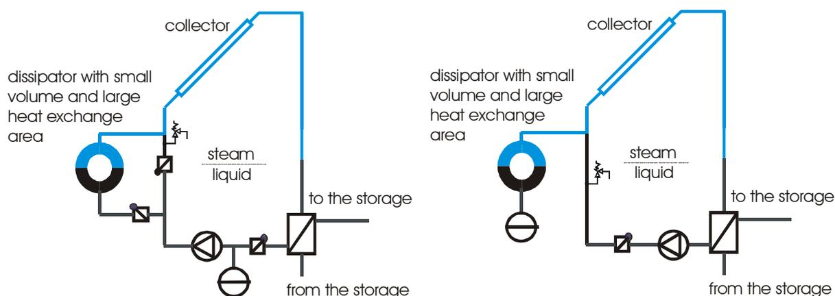
Figure 7: If the emptying behaviour of the collector cannot be improved, a simple automatically controlled air cooler in the primary solar circuit can limit the steam volume.
