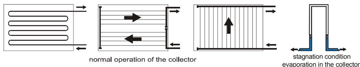
*Figure 4: Schematic examples of common collector circuitries with good emptying behaviour (the three schematics on the left illustrate the normal function of the collectors, while the right-hand schematic shows in simplified terms the condition of steam formation in the collector).*
