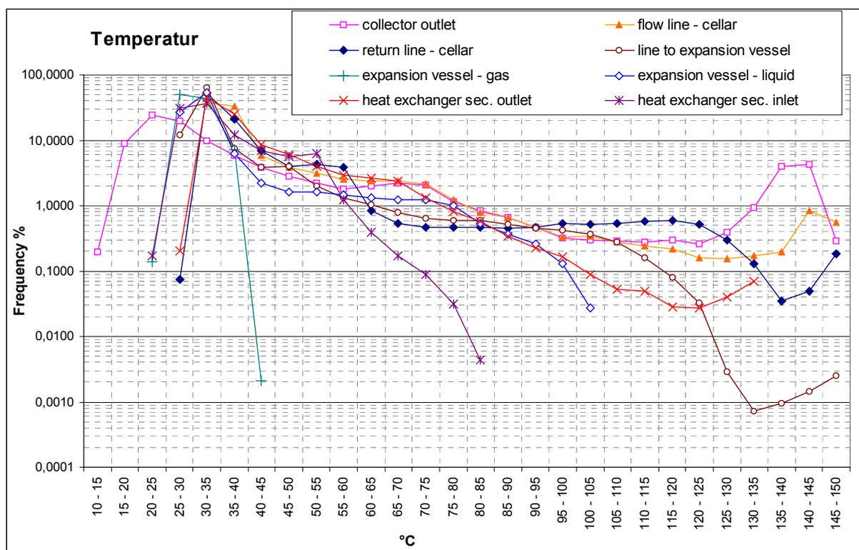
Figure 2: Measured example of frequencies of different system temperatures during a 5-months period (May to September) of a combisystem with a collector with poor emptying behaviour. A frequency of 1% corresponds to 36.7 h, 0.01% corresponds to 22 min.
