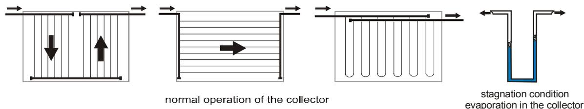
*Figure 3: Schematic examples of common collector circuits with poor emptying behaviour (the three schematics on the left illustrate the normal function of the collectors, while the right-hand schematic shows in simplified terms the condition of steam formation in the collector).*
