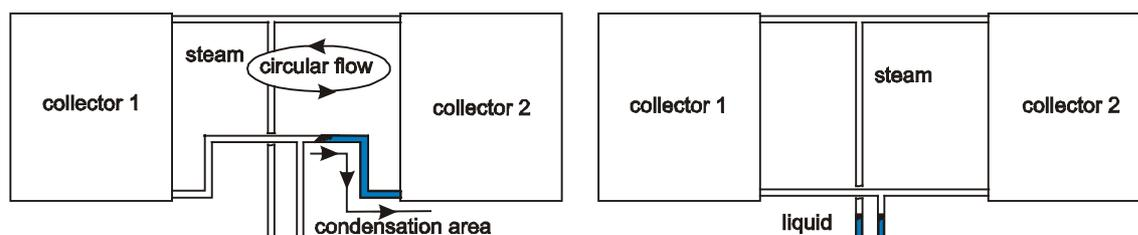
Figure 5: Examples of the interconnection of two collectors which empty well with poor emptying behaviour (left figure) and good emptying behaviour (right figure). The circular flow shown on the left-hand figure supplies liquid for a long period of time which leads to the further formation of steam in one of the collectors.
