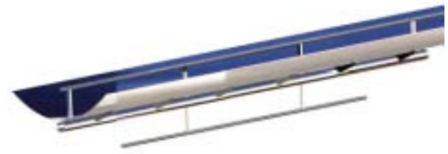
CAD model of the PolyTrough 1200
