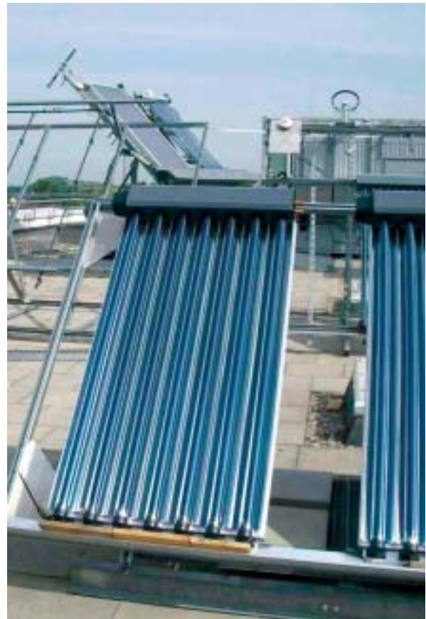
Evacuated tubular collector ESE VACOSOL installed on a test rig at Fraunhofer ISE
