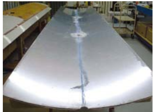
First panel from prototype tooling
