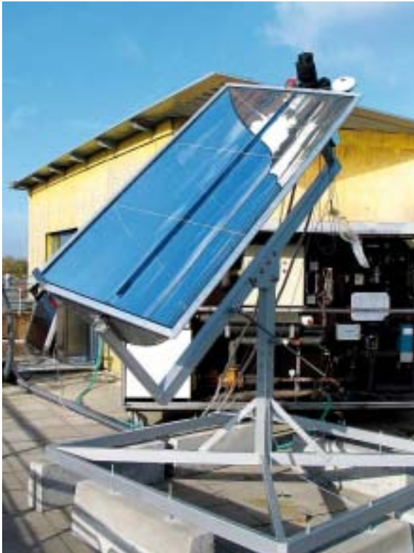
Testing of the PTC 1000 at the SIJ
