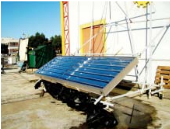
Prototype MAXI collector being tested at INETI
