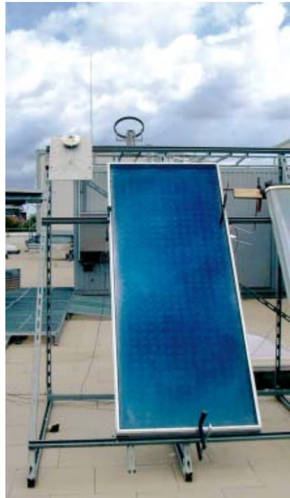
Double-glazed collector with AR-glass at Fraunhofer ISE's outdoor test site. The collector was built for first tests and comparison with a single-glazed collector (Collector components from Energie Solaire).
