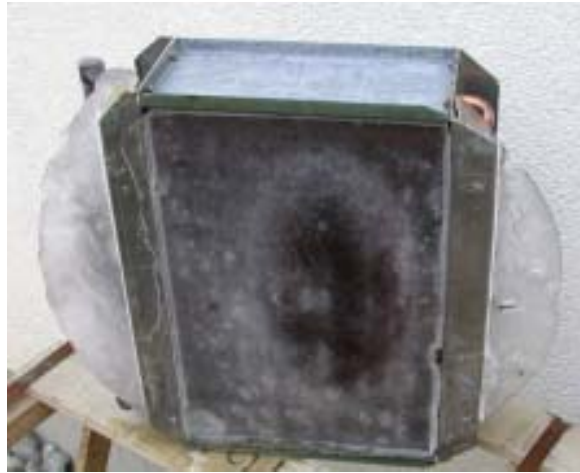
Fig. 35: Evaporator with frozen ice sheet which used to be the water surface
