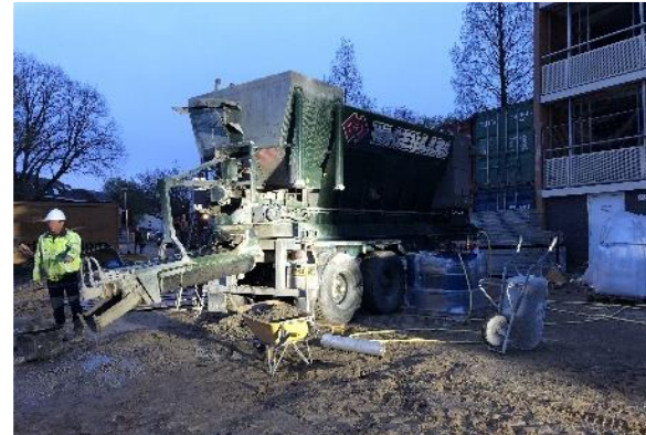
Mobile on-site factory for producing circular concrete
