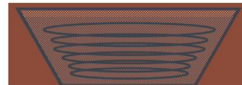
Soil-water pit thermal energy store (SW-PTES)
