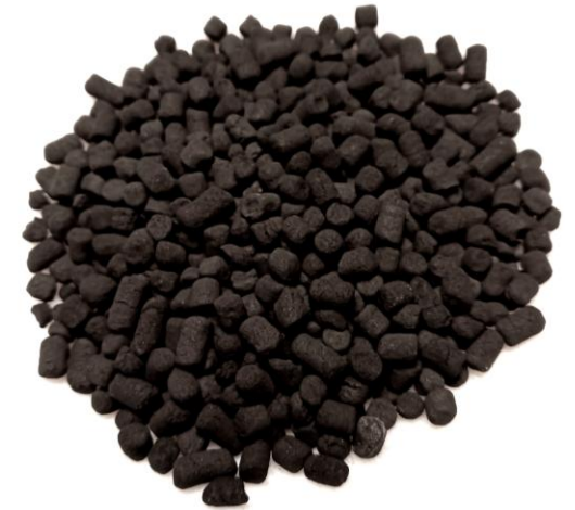
activated carbon impregnated with calcium chloride cylindrical grains from ~ 2 - 3 mm
