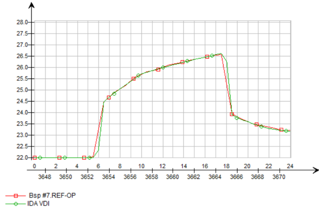
Figure 4: Comparison of operative temperature: IDA VDI model versus reference op. temperature according to VDI 6007, Test Case 7
